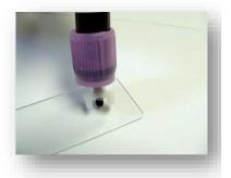
Hold the primary slide with the forefinger and using another slide as the upper slide, place the upper slide at a 30 degree angle halfway down the slide from the drop of blood.
