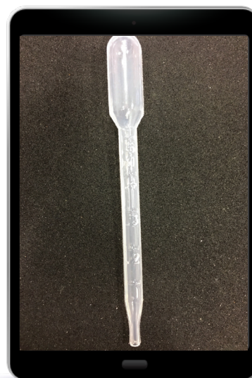
Transfer Pipette (with 0.1 mL [100 µL] graduations)
